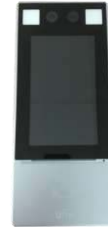
Temperature access control
